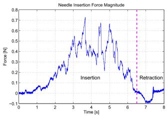
Fig. 2. Needle insertion and retraction forces into muscle tissue. At t = 6.5 s operator stops the insertion and quickly retracts the needle.
