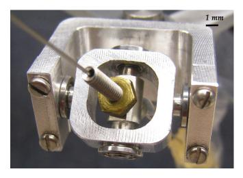
Fig. 6. 2 DOF Gimbal Mechanism: The needle can slide through the guide that is placed in the center.
